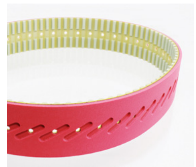
Sectional tooth removal - drive side, slotting and hole punch for vacuum
