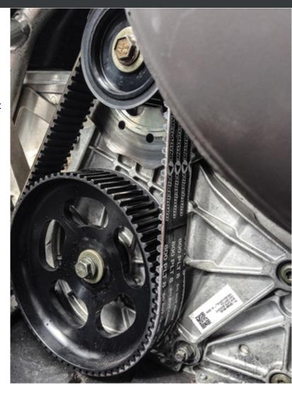
On misaligned drives, belts can roll or shift within the pulleys or throw the load to one side, stretching and damaging the belt. The pulleys will also wear unevenly, resulting in reduced lifespan. Angular misalignment can cause differential tension on the belt, wearing it out more quickly. Finally, bushings that have deteriorated or become loose can also affect alignment by causing the pulley to shift.
